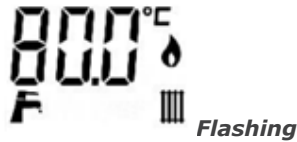
Radiator Symbol Radiator Circuit Temperature
